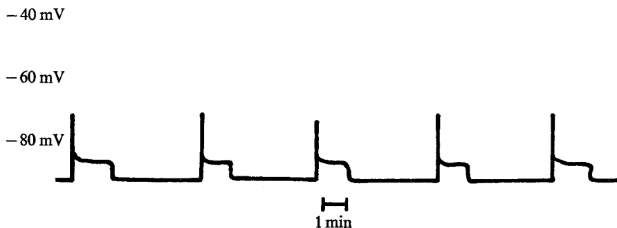
Fig. 3. Effect of the sudden change of the salt concentration. Spontaneous firing of the emf across the membrane. Initial salt concentration, 1 mM/1 mM KCl. Final salt concentration, 7.8 mM/62.5 mM KCl
